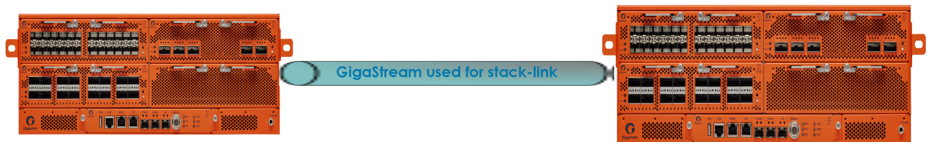
Figure 4 Daisy-Chain Configuration using GigaStream for Stack-link
